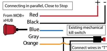
MOB+ Wireless Kill Switch can be installed together with your existing kill switch by connecting it in series or parallel. If you should connect in series or parallel depends on your existing kill switch function. The above picture shows an example with Close to Stop connection.
